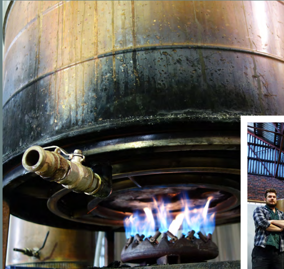
Top left: Rustic, direct-fired pot still like the moonshine stills of old; Bottom right: Whipper Snapper Distillery, Perth
